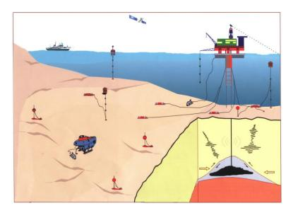
Figure 1. A general structure of the coastal zone geophysical hazard observation system based on drilling platforms
