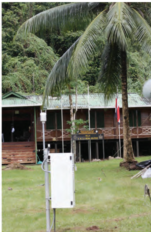
Fig. 3. ISCO CGPS monument at Wafer Bay (left). Box containing GPS receiver, met package, radio link and power supply (right).
