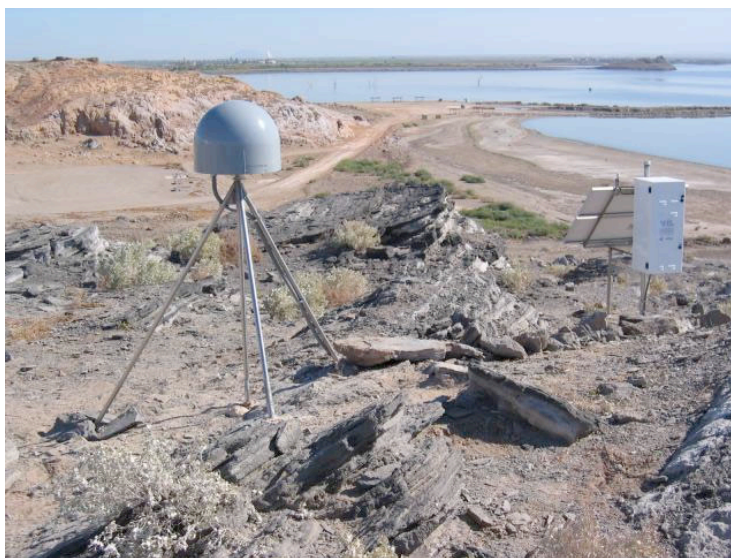
Figure 6. A short-drilled braced monument (SDBM) installation in the EarthScope network. A similar monument and station configuration is proposed for COCONet.
