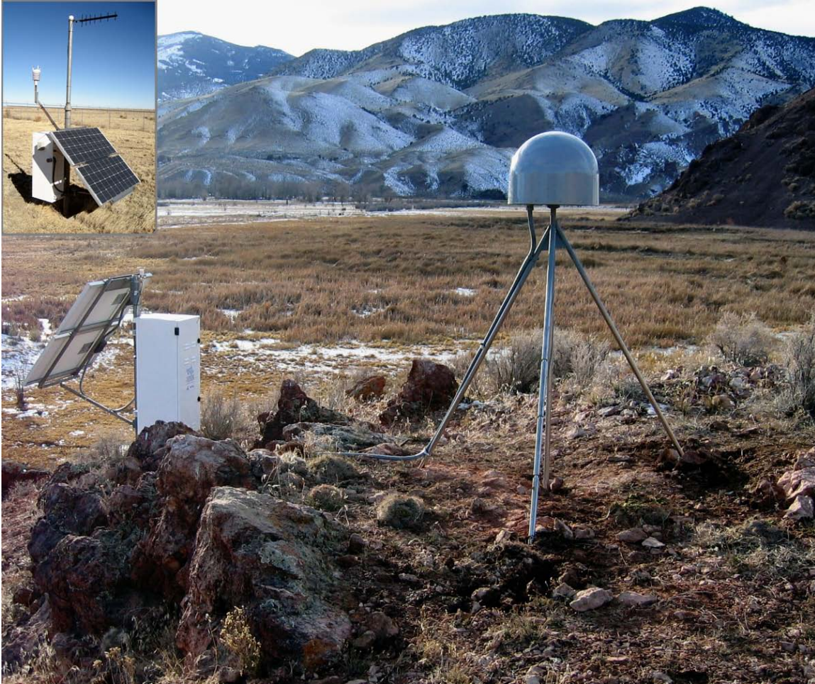
Figure 1. PBO station P009 near Marysvale, Utah. This station combines a short drilled-braced monument with a radome housing the geodetic antenna (right) and the receiver and data communications enclosure and solar panels (left). A similar monument style will be utilized on COCONet where competent bedrock exists. Other monument options include building mounts and concrete pillars where there is no suitable bedrock. Inset illustrates a met pack installation.
