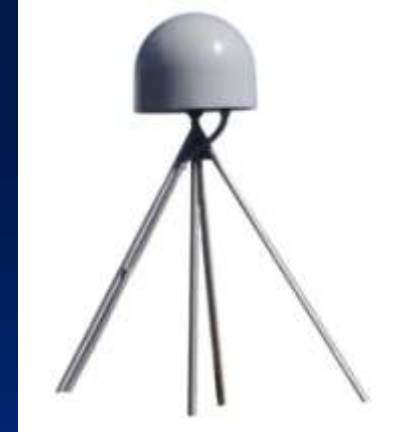
Short Drilled Braced GPS Monument
